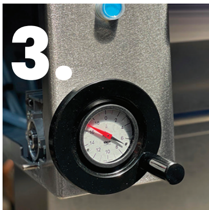
The handwheel on the machine allows the operator to change the skinning depth quickly and easily.
