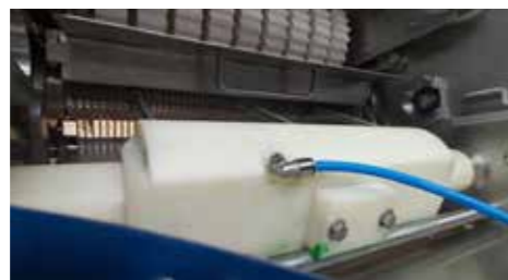
Travelling blower ensuring optimal skinning roller efficiency
